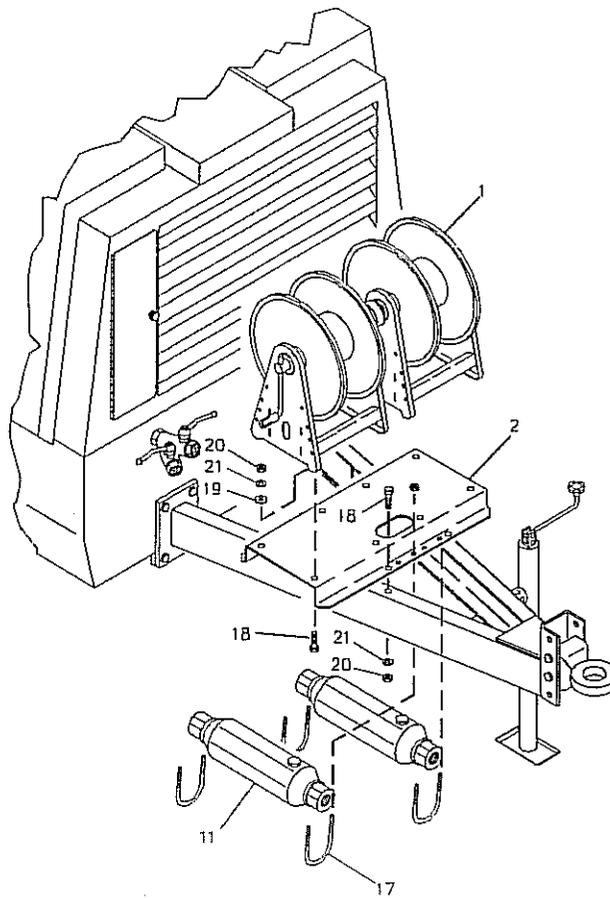
ASSEMBLY OF HOSE REELS AND LINE OILERS
